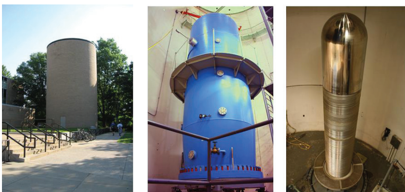
Figure 1. Three views of the UKAL accelerator facility: (left) the silo in which the accelerator is housed on the University of Kentucky campus; (middle) the accelerator with tank on; and (right) the accelerator with the tank removed and the resistor column and terminal visible.
