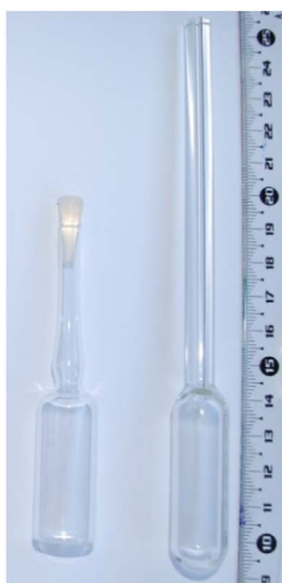
Fig. 1. BIPM ampoule used for liquid (on the left) and for gas (on the right).
