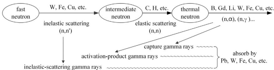
Fig. 1. Main interactions considered in the shielding of fast neutrons.
