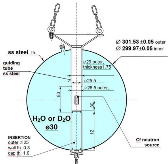
Fig. 1. Light or heavy water sphere design with neutron source. All dimensions shown are in mm. The spheres were hung up to a distance of 2 m from the floor to minimize the room effect.
