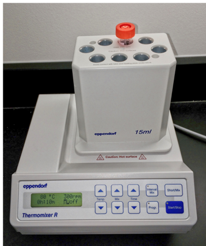
Fig. 1. Eppendorf Thermomixer fitted with the heating element for a 15-mL centrifuge tube. In our initial manual synthesis method, a single-use sterile centrifuge tube containing the [ ^{68}\text{Ga} ]Ga-DOTA-NOC reaction solution was simply heated in the 80 °C thermomixer with swirling at \geq 300 rpm for 10-min to complete the labeling reaction (with the apparatus shielded within > 5 -cm walls of lead bricks).
