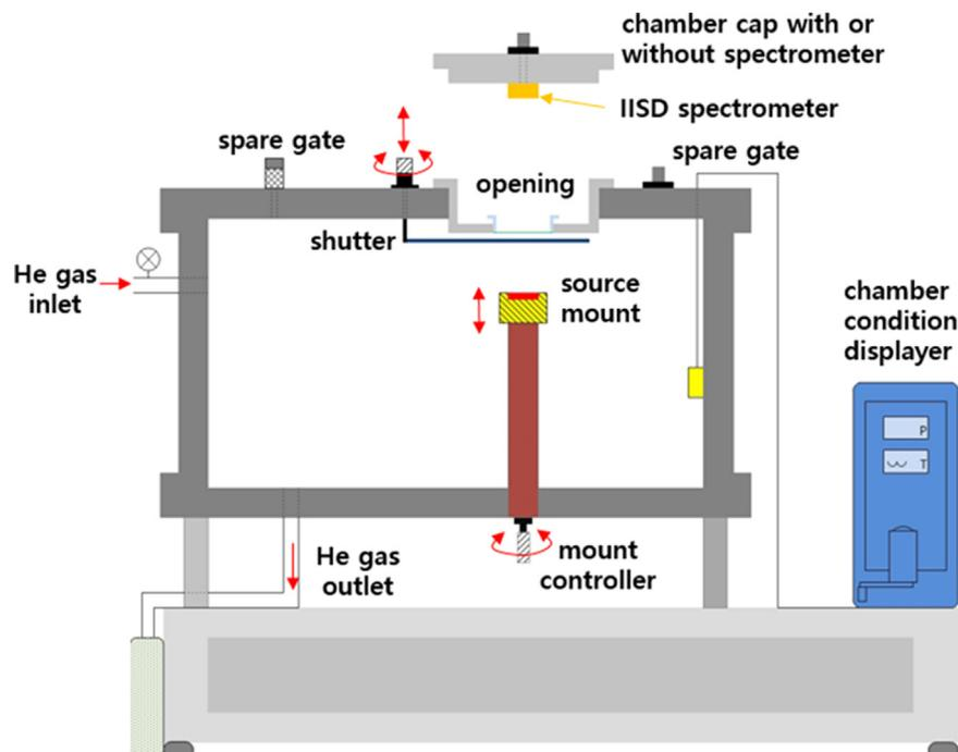
Fig. 1. Schematic of the SNU alpha particle irradiator.
