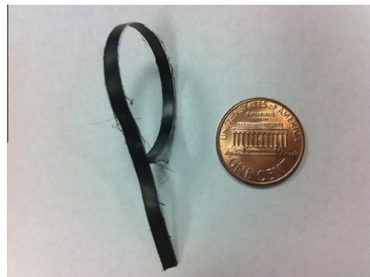
Fig. 3. A photograph of the flexible CNT/nylon 6,6 composite film (before stretching) made by the drawing and winding method.
