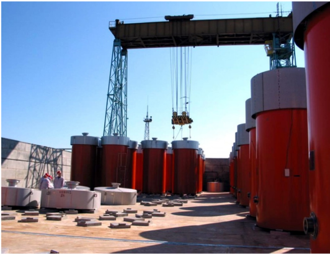
Fig. 1. CASTOR ® RBMK-1500 (on the left) and CONSTOR ® RBMK-1500 (on the right) storage casks in existing SNFSF at Ignalina NPP (Ignalina Nuclear Power Plant, 2016).
