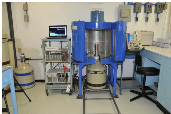
Fig. 1. Gamma-ray spectrometry system located at ININ's RSL. The picture shows the HPGe-detector, Dewar, shield, electronic items and computer with Gamma-vision software.
