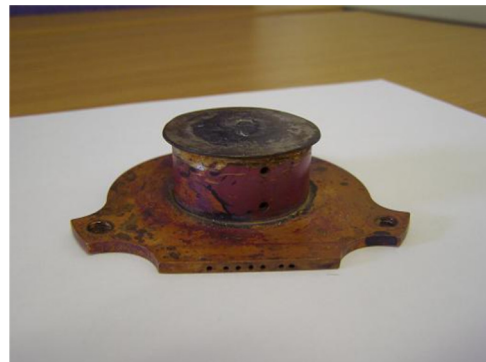
Fig. 2. Target blank prepared for induction heating.
