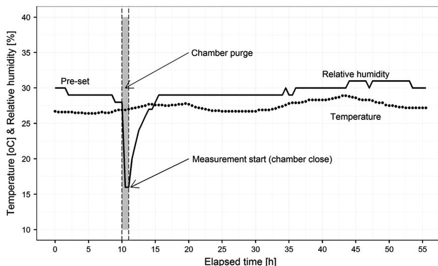
**Fig. 2.** Changes of relative humidity and temperature in the accumulation chamber during measurements.
