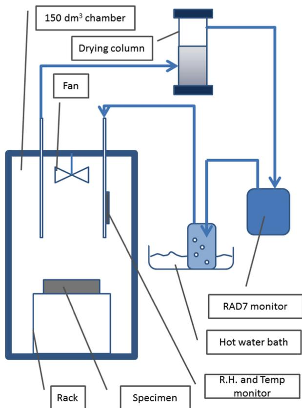
**Fig. 1.** Schematic of the system for exhalation rate measurement.
