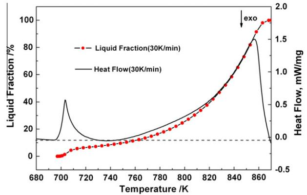
Fig. 1. DSC and liquid fraction curves of the as-cast C<sub>fiber</sub>/AZ91D composite.
