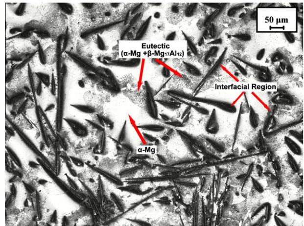
Fig. 2. Microstructure of the as-cast C<sub>fiber</sub>/AZ91D composite.
