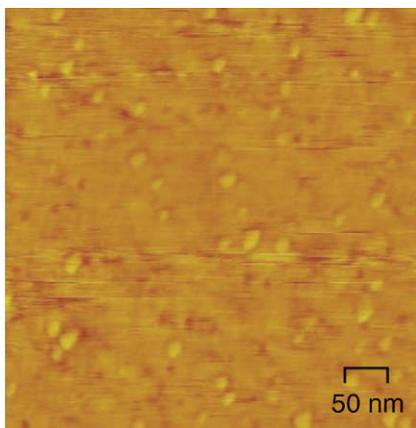
Fig. 1. Tapping-mode atomic force micrograph of 10 wt.% silica nanoparticle-modified bulk epoxy polymer.
