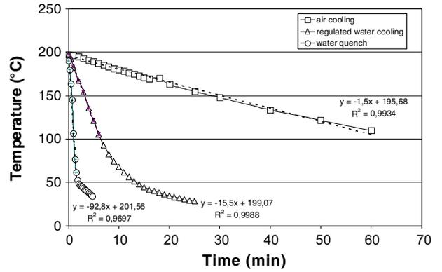
Fig. 2. Cooling kinetics for biocomposites.
