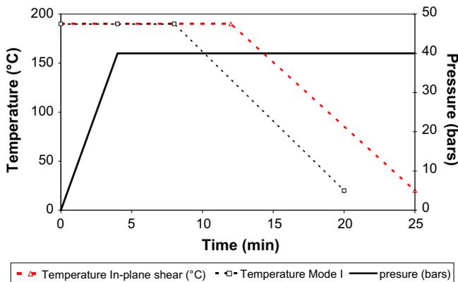
Fig. 1. Film stacking manufacturing cycle for in-plane shear and mode I specimens with water cooling ( $\sim 15.5^\circ\text{C}/\text{min}$ ).
