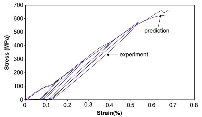
**Fig. 3.** Example of stress–strain curves predicted using the model for  $P_{Mi} = 0.5$ ; and obtained experimentally (C/SiC minicomposite) [16].
