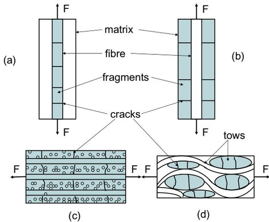
**Fig. 1.** Schematic diagrams showing examples of multiple cracking in various composite systems: (a) fiber fragmentation in a polymer matrix composite, (b) matrix fragmentation in a ceramic matrix composite, (c) in a cross ply laminate, (d) fragmentation of transverse tows in a woven composite.
