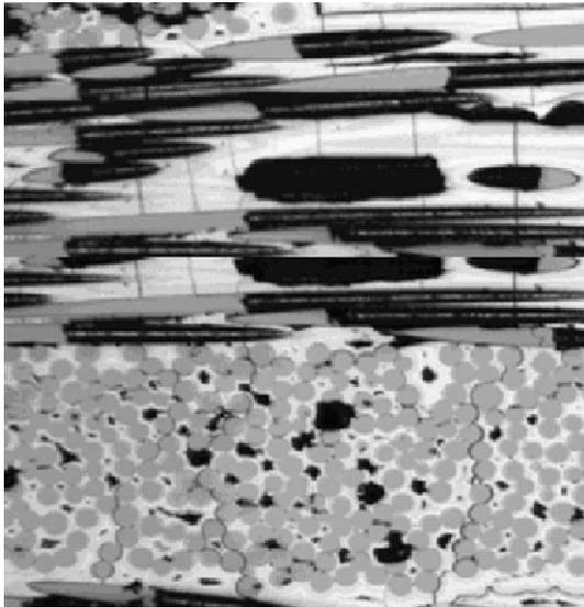
**Fig. 2.** SEM micrograph showing multiple cracks in the matrix of longitudinal tows, and of transverse tows of a woven ceramic matrix composite. Note that the cracks propagated through the tows.
