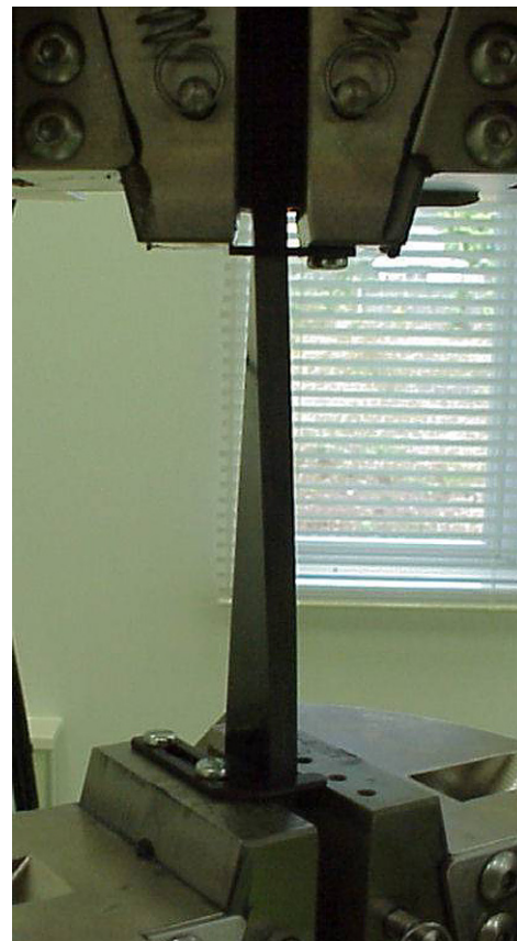
Fig. 1. Unidirectional CFRP specimen subjected to axial torsion.
