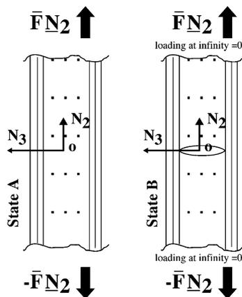
Fig. 1. Cross-ply laminate in traction (A being the healthy state, B the cracked state).
