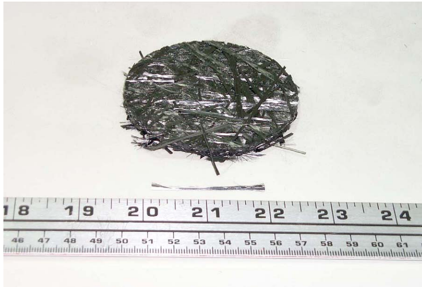
Fig. 1. A photograph of a dry preform of a chopped strand mat.
