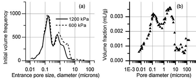
**Fig. 1.** (a) Comparing intrusion volume frequency ratios of samples compacted at the same water content and different vertical stresses [18], (b) pore-size distributions (PSD) of a clayey till subjected to 840 kPa of suction [19].
