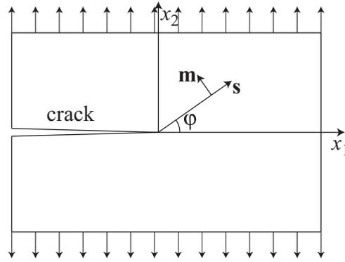
Fig. 1. The plane strain crack problem for single crystal.
