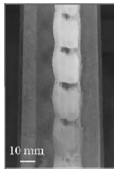
Fig. 2. (Extract from Saulot, 2005) Heavy corrugation of a rail.
