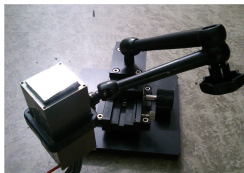
Fig. 2. Alpha-particle imaging detector supported by a flexible arm stand.
