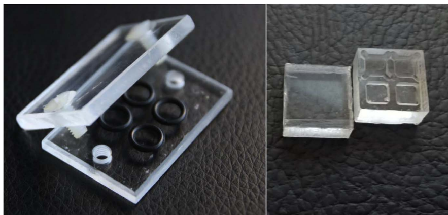
Fig. 1. Left frame: PMMA Holder No. 1 with two rubber O-rings for the NaCl and two for the LiF chips. Two nylon screws were used to tighten the PMMA plates together and to avoid any moisture from entering the dosimeter cavities. Right frame: PMMA Holder No. 2, with two cavities for the NaCl and two for the LiF chips.
