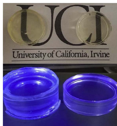
Fig. 1. PVT-PPO/QD (left) and PVT-PPO (right) samples, bottom picture shows the luminescence under UV lamp excitation at around 250 nm.
