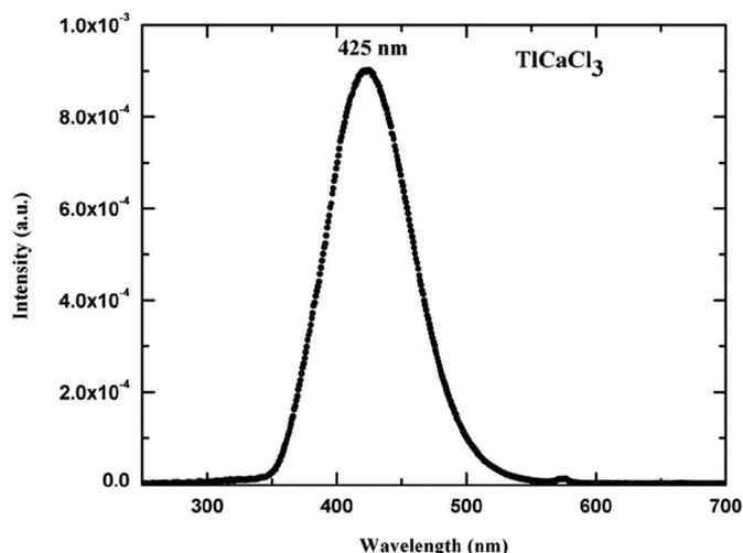
Fig. 2. Emission spectra of  $\text{TlCaCl}_3$  crystal recorded under x-ray irradiation at room temperature.
