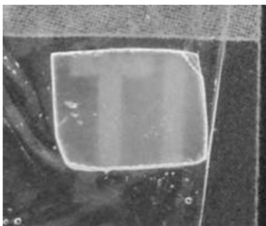
Fig. 1. A polished sample of the as grown  $\text{TlCaCl}_3$  crystal.
