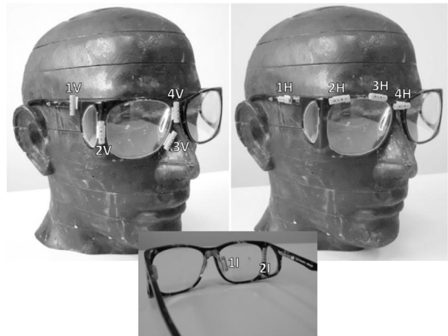
Fig. 2. Positions where RPL dosimeters were placed, over and under the shielding of lead glasses.
