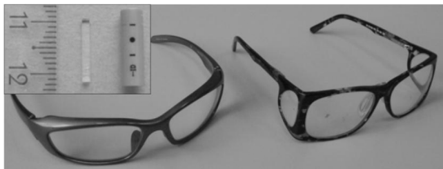
Fig. 1. Models of lead glasses used. In detail, RPL glass dosimeter GD-352M.
