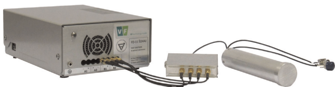
Fig. 1. Two-parametric digital spectrometric system. From the left side: digital spectrometer, amplifier and detector with HV connector.
