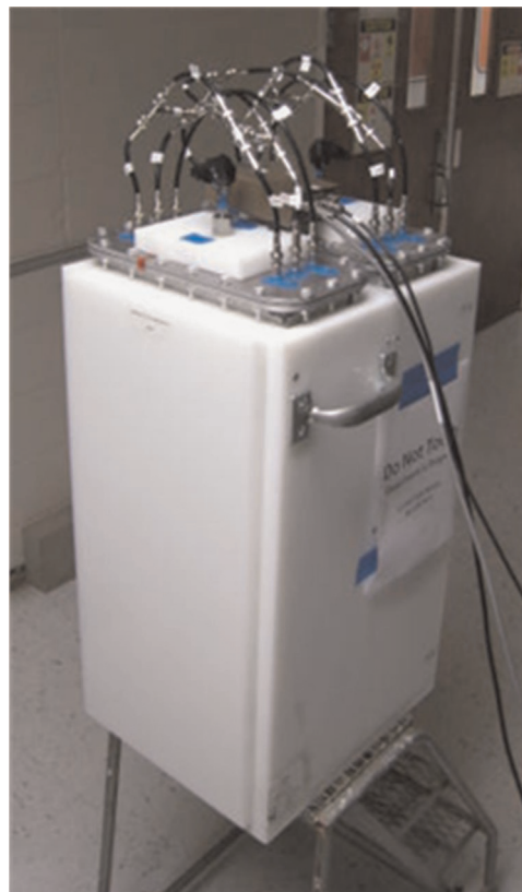
Fig. 1. The arrayed detection system containing the two Li foil MWPCs and HDPE neutron moderator. The “Front” is to the left; the handle is on one “Side”.
