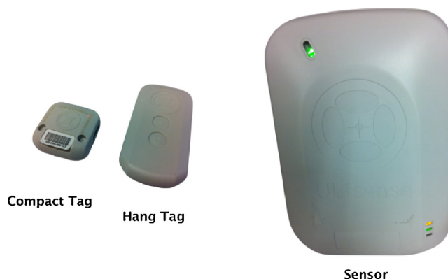
Fig. 1. Real-time locating sensor (mounted in the corners of ceilings) and two tags used in the study (a wrist “compact tag” and “hang tag” which can be worn around the neck). The tags emit an ultra-wide band radio signal that is triangulated by multiple sensors in the environment. The tags are worn by residents to track their location and movement in real-time.
