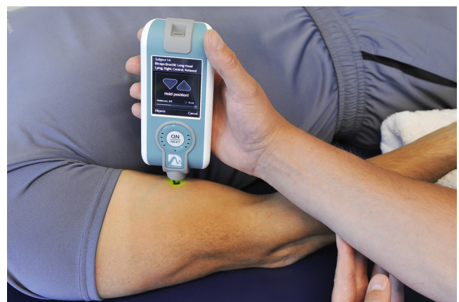
Fig. 1. MyotonPRO technique for measurement of biceps brachii (BB) stiffness, tone and elasticity.
