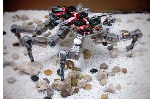
Fig. 1 The hexapod robot HITCR-II walking on unstructured terrain.
