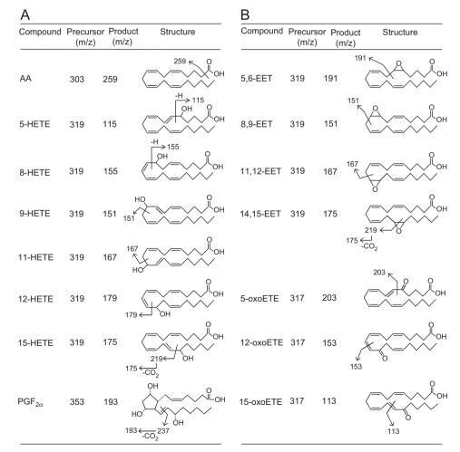
**Fig. 1.** Precursor ion  $\rightarrow$  product ion transitions and suggested structure of the major product ion derived from each eicosanoid. ESI negative-ion full scan was used for identification of precursor ions for each of the analytes and ESI negative-ion product scan was used for identification of the specific product ions from each of the precursors. Suggested structures consistent with the product ions produced are depicted for each analyte.
