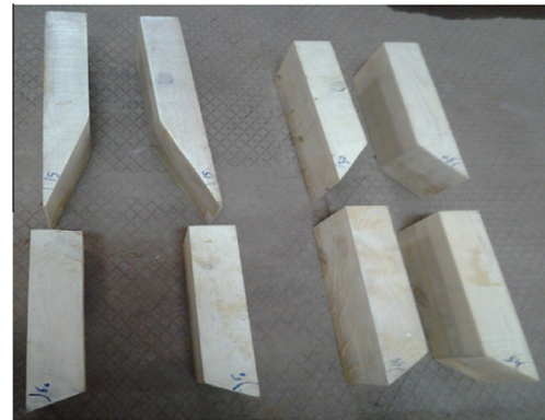
Photo 2 Different shapes of abutment.
