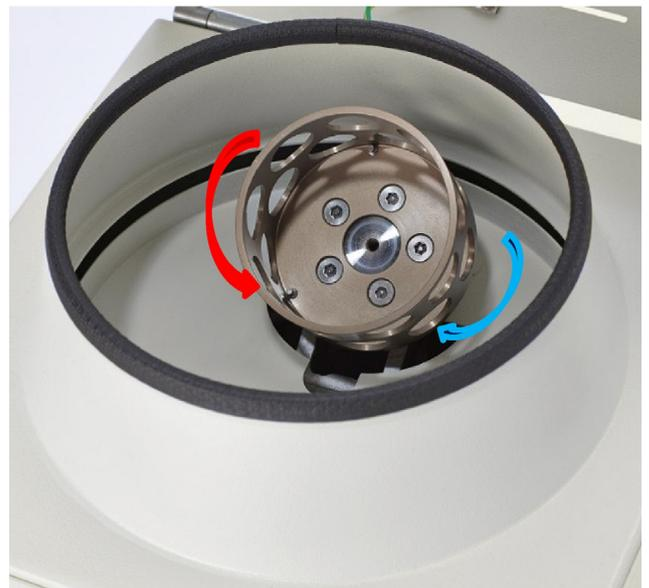
**Fig. 1.** A photo showing the new powder mixing machine used in the current study. The arrows show the rotation of bottom plate and the basket along their axes in different directions.
