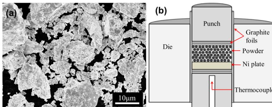
Fig. 1. (a) SEM micrograph of hand-ground *n*-type PbTe fine powder, showing particles smaller than 10  $\mu\text{m}$ ; (b) schematic illustration of the experimental set-up in SPS.
