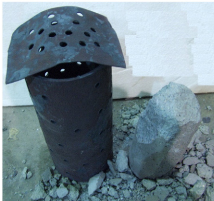
Fig. 1. Spalled UHSC specimens without fibers.
