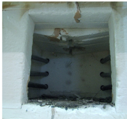
Fig. 1. Spalled UHSC specimens without fibers.
