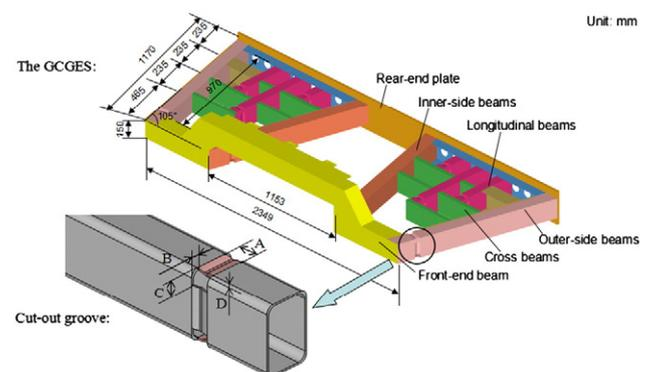
Fig. 1. The GCGES with detailed cut-out grooves for subway vehicles.
