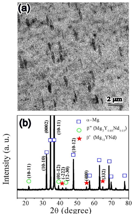
Fig. 2. (a) TEM image and (b) XRD patterns of the AA sample heated at 510 °C for 5 min before hot deformation.
