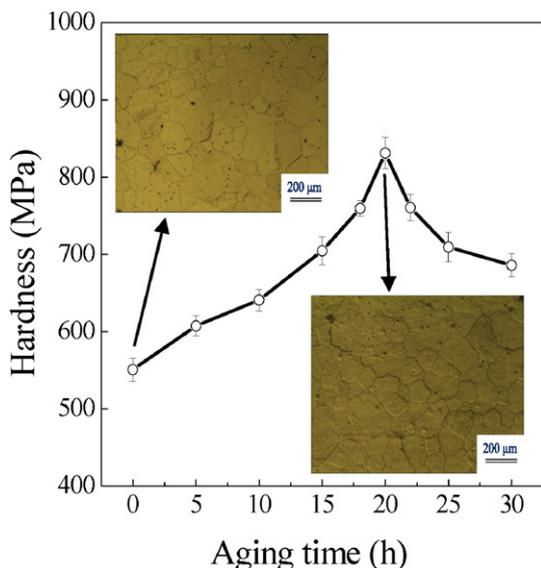
Fig. 1. Hardness curves and typical microstructures of Mg-4Y-2Nd-0.2Zn-0.5Zr alloy treated in solid solution and peak aging at 220 °C.
