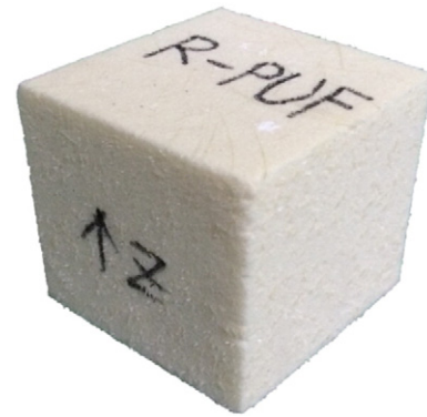
Fig. 2. Photograph of RPUF test specimen for compressive test.
