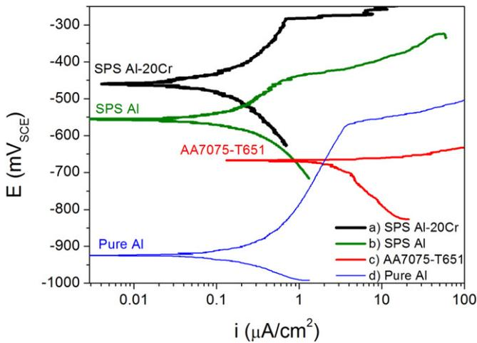
**Fig. 1.** Representative potentiodynamic polarization curves for spark plasma sintered a) Al-20 wt.% Cr and b) Al alloys along with c) AA7075-T651 and d) pure wrought Al in 0.01 M NaCl.
