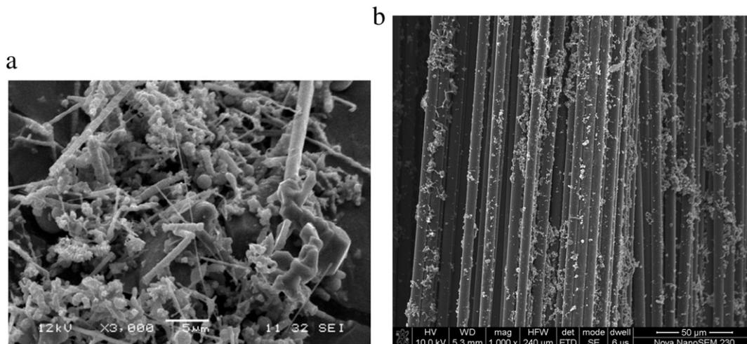
Fig. 2. SEM images of SiCNFs and the carbon fibers covering with SiCNFs (a) SiCNFs (b) Carbon fibers covered by SiCNFs.
