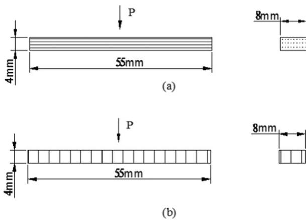
Fig. 1. Flexural test geometry (a) vertical direction; (b) parallel direction.
