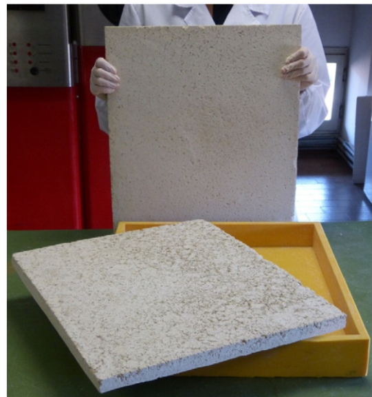
Fig. 1. Example of geopolymer–vermiculite panels of 55 cm × 47 cm × 3 cm.
