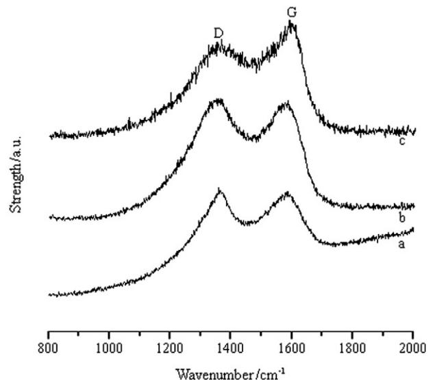
Fig. 3. Raman curves of fibers carbonized at three different temperatures: (a) 400 °C; (b) 700 °C; and (c) 1000 °C.
