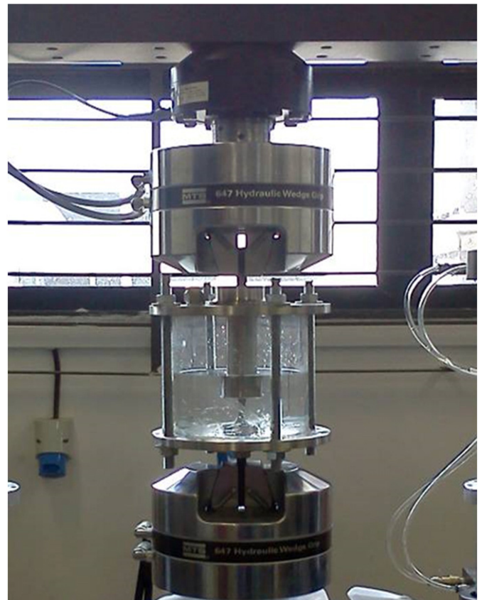
Fig. 2. Chamber assembled for the corrosion-fatigue test.
