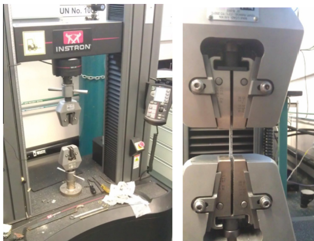
Fig. 1. INSTRON hydraulic machine for low-speed test.
