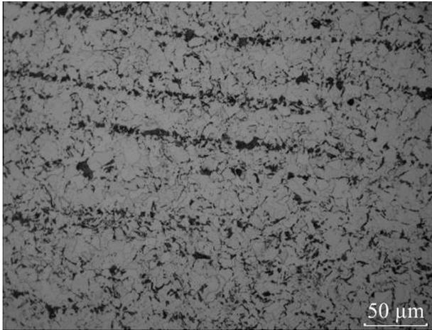
Fig. 1. Optical micrograph of the base metal E40 steel.
