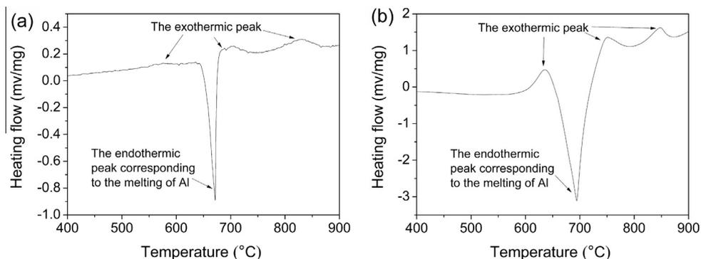
Fig. 1. DSC curves of Al–20 wt%CuO samples obtained under flowing argon using heating rates of (a)  $5\ ^\circ\text{C}/\text{min}$  and (b)  $50\ ^\circ\text{C}/\text{min}$ .
