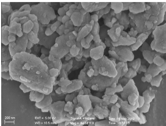
Fig. 2. SEM morphology of Ti 3 SiC 2 powders.
