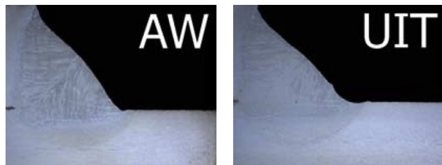
(a) Cross-section of an as-welded weld toe [6]
