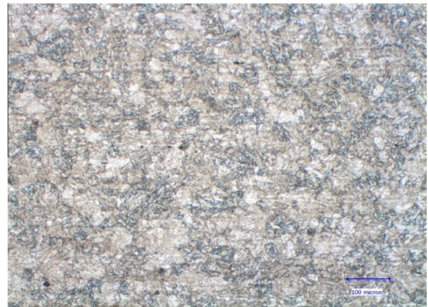
Fig. 1. Toolox 33 ® martensitic microstructure, 100×.
